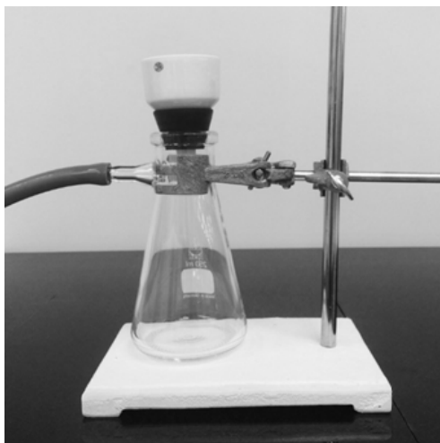
Figure 2: Set up needed for suction filtration.
