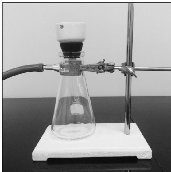
**Figure 2:** Set up required for suction filtration.
