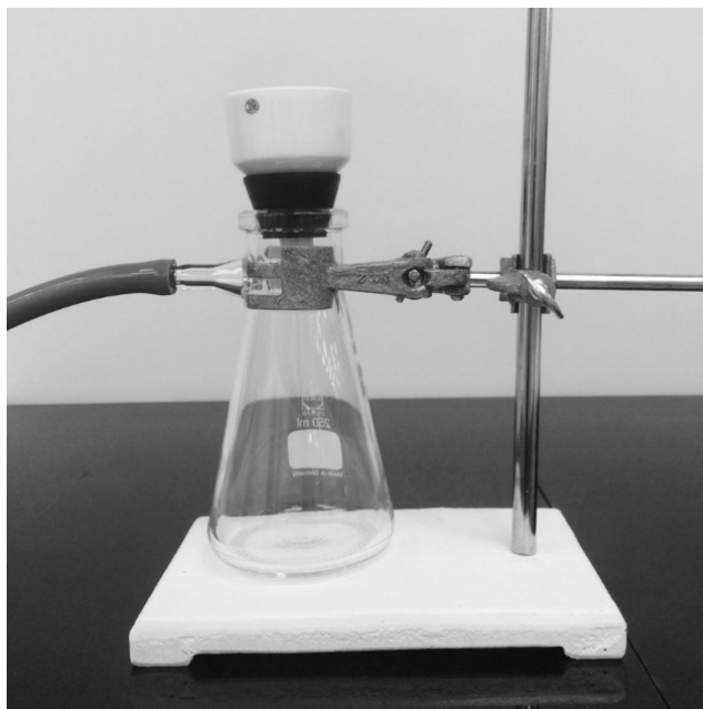
Figure 2: Set up needed for suction filtration.
